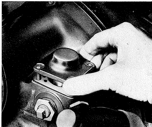
Figure 35—Removing Gun Synchronizer Pad Cover
