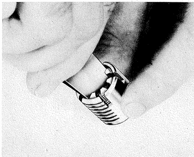
Figure 44—Adjusting Positive High Pitch Adjusting Screw
